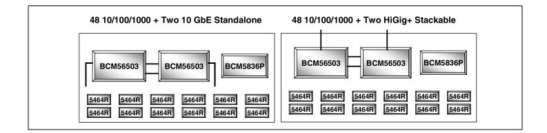
The BCM56503 is the fifth generation of the highly-integrated and costeffective StrataSwitch and StrataXGS product line. The BCM56503 is a single-chip solution with 24-GbE ports, and three 10-GbE/HiGig+ uplink ports.
